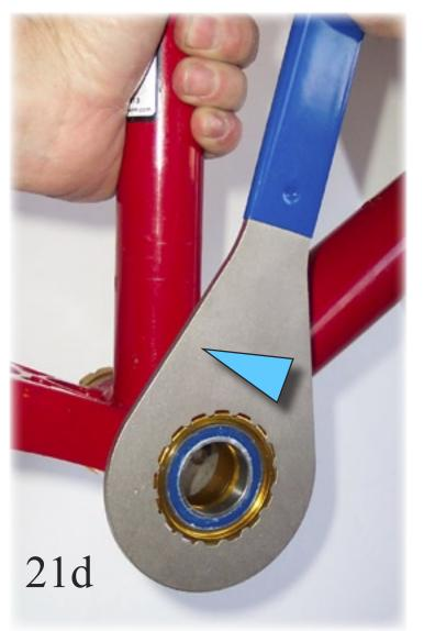
22) Although the bearing is sealed, you may wish to apply a layer of Super-Web Grease® for extra protection.
