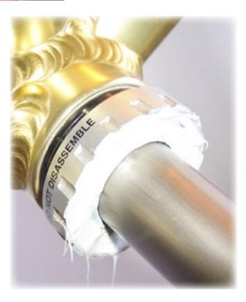
25) Insert the right crank assembly. If your bike's bottom bracket faces are parallel and the bearings are properly seated, the spindle should line up with the opposite bearing and come through with very little effort. If the spindle tightens up at the last few millemeters, you may lightly tap the drive side with the rubber-faced mallet.
