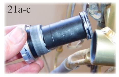
21) Re-install the right, or drive side cup and spacer(s).
