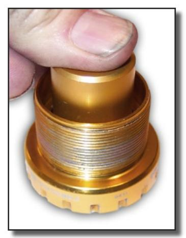
9) Apply pressure to the Collet Expander until it "seats" between the collet halves.
