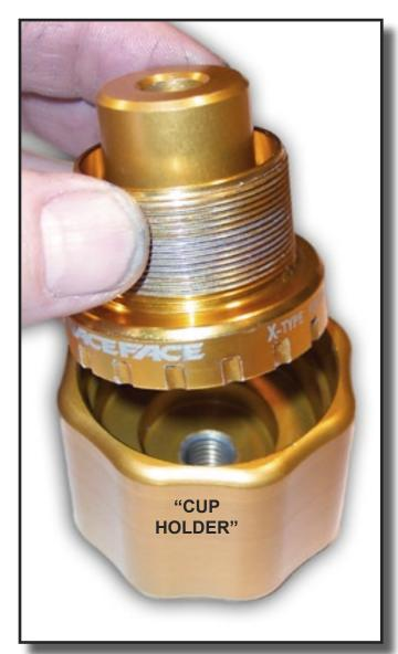
10) Set the bearing cup (with collet and expander) into the Cup Holder.
