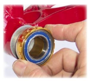
c) Start the cup into the frame by hand. The left side threads in normally (clockwise).
