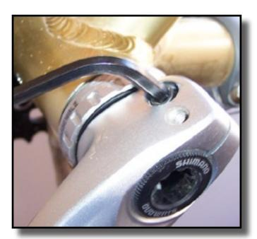
1) Loosen the left-side crank arm bolts using the 5mm Allen wrench. Loosen them in an alternating pattern.
