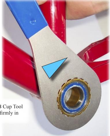
d) Use a proper BB Cup Tool to tighten the cup firmly in place.
