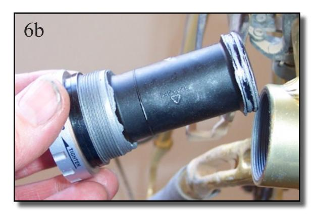
b) Set the inner sleeve and the spacers aside (take note of the spacers for proper re-assembly).
