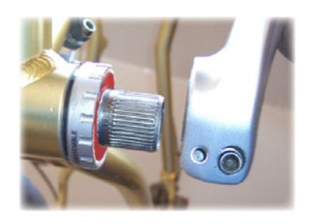
27) Lubricate the axle splines and push the left crank arm onto the axle (the crank arm will only slide on if it is aligned correctly--notice the one wide groove).
