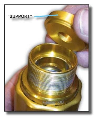
18) Place the Support into the threaded end of the bearing cup.
