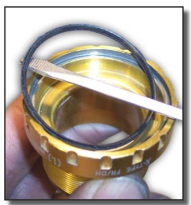
14) Remove the sealing ring from the outer circumference of the bearing cup.
