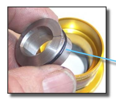
7) Set one of the bearing cups down on a flat surface and insert the Collet from the Bearing Puller/Press Tool.
